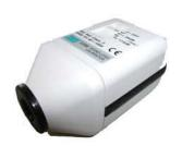
The 1356 is a portable sound level meter calibrator for use with the 1351 sound level meter. This calibrator conforms to ANSI S1.40-1984 and IEC942 1988 Class 2 and provides 2 calibration levels of 94dB and 114 dB.
