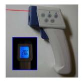
The CHY 111 is a portable easy to use 3½ digit, compact sized digital infrared thermometer with laser sighting for simple one hand operation. Features include, backlit LCD display, auto-hold function, auto powerdown, adjustable emissivity and Celsius/ Fahrenheit selectable. Temperature scale is -30°C to 550°C (-22°F to 1022°F). 10:1 Field Of View.
