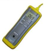
The 305P is a portable 3½ digit, compact sized digital thermometer designed to use external K-Type thermocouples as the temperature sensor. Temperature indication follows the National Bureau of Standards and IEC 584 temperature/voltage tables for K-Type thermocouples. Celsius or Fahrenheit user selectable. Temperature scale is -50°C to 1300°C (-58°F to 2000°F)
